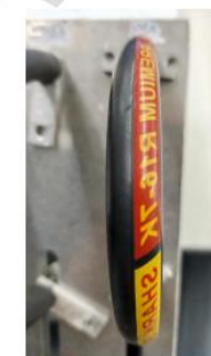
Fig. 6 – Photo of the sample A 704 after 600h on ozone chamber
